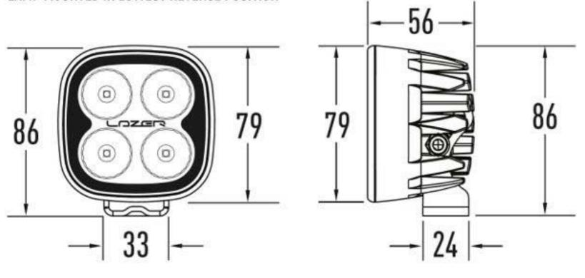
MEASUREMENTS IN MM
